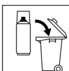
The completely emptied spray cans must be disposed of in the recycling system. Cans with hardened material must be disposed of as special waste.
